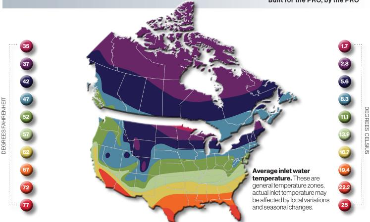
Use your location on the map to correlate with legend for average ground water temperature in the U.S. and Canada. For Hawaii and Puerto Rico, use ground water temperature of  $75^{\circ}$  F /  $23.9^{\circ}$  C.
